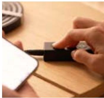
On the Wi-Fi dimmer box, press and hold both brightness+ buttons at the same time for 5 seconds. The LED strip lights will flash five times to show that it's ready to be paired.
