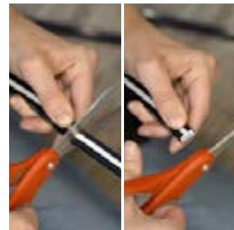
**Before cutting your lights, unplug the power supply from the wall.** Using sharp scissors with a 4" blade (the size of your standard office scissors), carefully cut on a dark node, as straight as possible, completely through the strip. Finish the cut end with a black silicone end cap (supplied in box).
