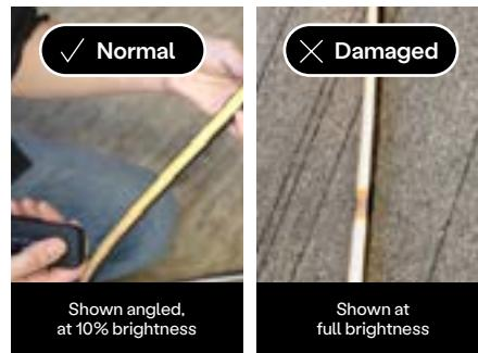
Check all lights. It is normal to see some smaller, faint dark spots as the lights are unrolled and flattened for the first time. A large, dark spot indicates a light is damaged.
